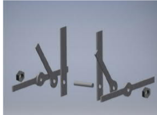
Image 9: Model of a Disassembled Pin Connection
